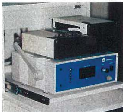
Figure 3—The modified sulfide monitor (Halimeter™) (below) and the pen-writer (above) used for measuring VSC.
